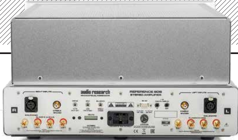
ABOVE: Small toggles switch between single-ended (RCA) and balanced (XLR) inputs, fan speed and auto-shut off (signal sensing). Tube hours are indicated beside a bladed IEC mains inlet, while 4mm speaker binding posts offer 16ohm, 8ohm and 4ohm taps
